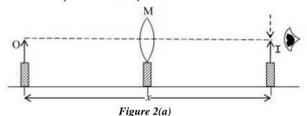
(ii) Arrange the object pin O, the image pin I and the lens M on the optical bench or table top as shown in *Figure 2(a)* so that the tips of O and I lie on the principal axis of the lens.
